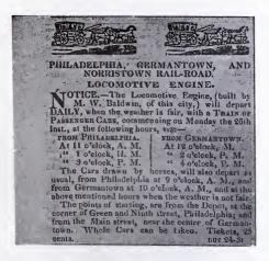
This announcement did not mean that in wet weather horses would be attached to the locomotive to aid it in drawing the train, but that the usual horse cars would be employed in making the trips upon the road without the engine.
