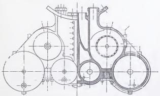
CROSS SECTION OF BALANCED COMPOUND CYLINDERS
